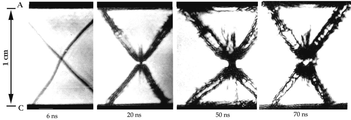
**Fig. 1.** The main stages of X-pinch dynamics are shown with schlieren images.
