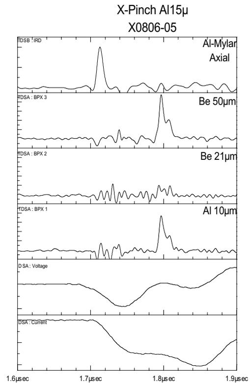
**Fig. 3.** Sample of emission signals, plus current and voltage monitoring.
