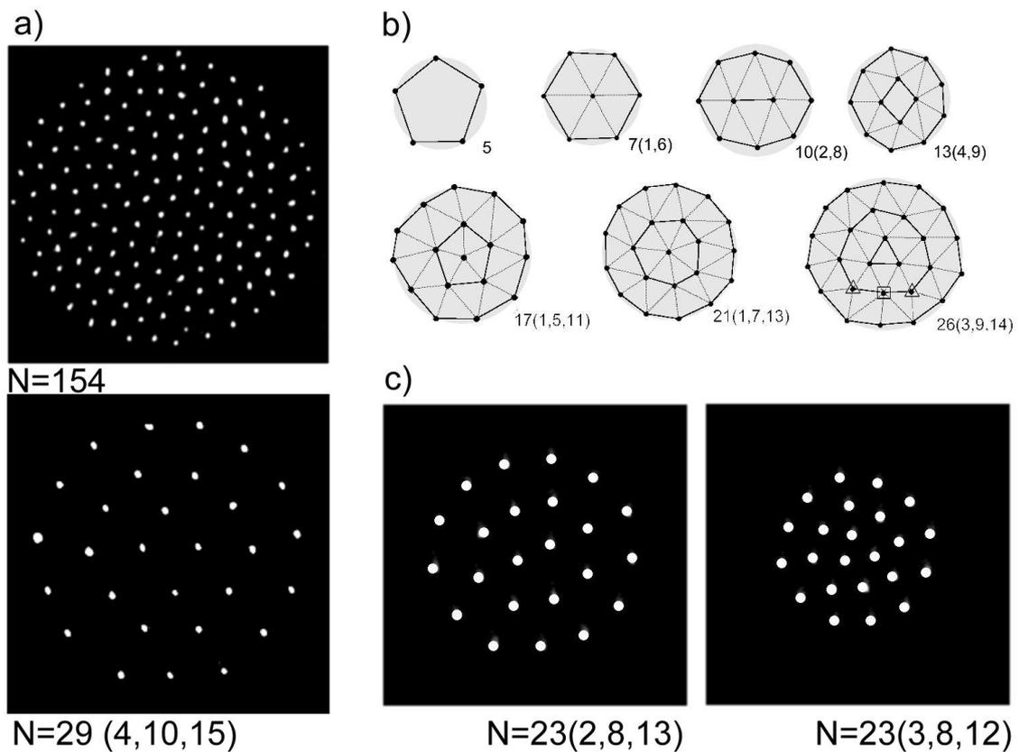
**Fig. 1.** a) The typical microimages with large and small  $N$  from our experiment. b) The stable triangulated configurations obtained from our experimental images. The scales are not exactly the same. The mean interparticle distance is about 0.6 mm. c) The typical ground state configurations from the MD simulation using bare Coulomb interaction. Making the Debye length too short will turn the  $(2,8,13)$  structure into the  $(3,8,12)$  structure which has less elongated shape.
