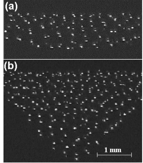
**Figure 2.** Images of dust cloud (side view). (a)  $V_c = -15 \text{ V}$ ,  $V_r = -20 \text{ V}$ , (b)  $V_c = -15 \text{ V}$ ,  $V_r = -30 \text{ V}$
