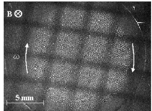
**Figure 3.** Image of rotational motion of dust particles observed through a mesh cathode from the top
