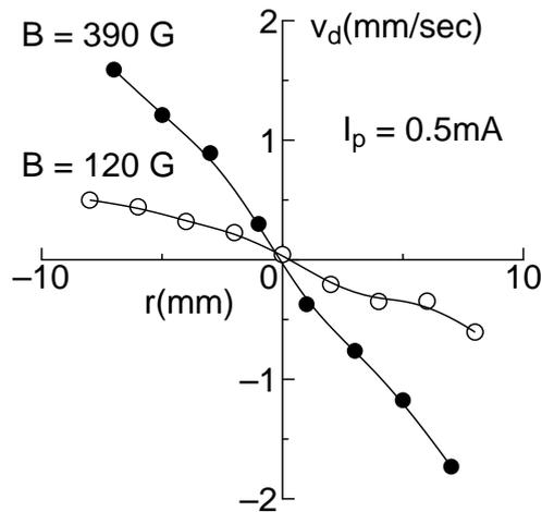
**Figure 5.** Radial profiles of particle rotation velocity  $v_d$  under magnetic fields of  $B = 120$  G ( $\circ$ ) and  $390$  G ( $\bullet$ )
