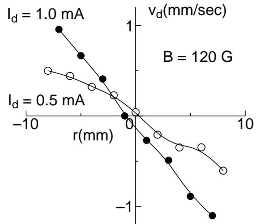
**Figure 6.** Radial profiles of particle rotation velocity  $v_d$  for discharge currents of  $I_d = 0.5$  mA ( $\circ$ ) and  $1.0$  mA ( $\bullet$ )
