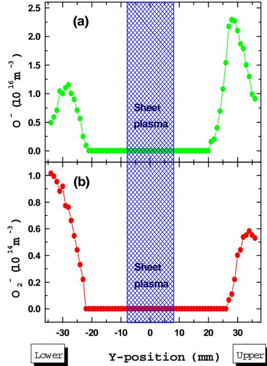
**Fig. 2** The spatial profiles of (a)  $O^-$  and (b)  $O_2^-$  is plotted against the y-direction of the width of the sheet plasma.
