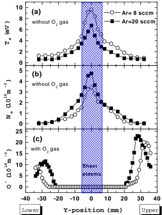
**Fig. 3** The spatial profiles of (a) the electron temperature  $T_e$ , (b) the electron density  $n_e$ , and (c) the density of  $O^-$  are plotted against the y-direction of width of the sheet plasma.
