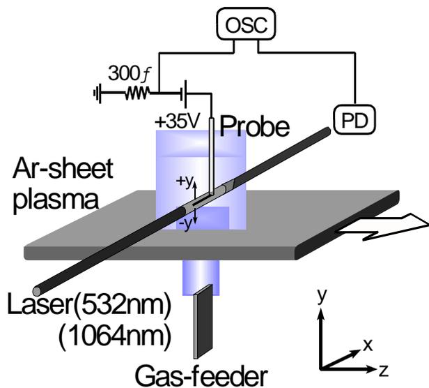
Fig. 1. Schematic diagram of the magnetized sheet plasma crossed with the vertical gas-flow system.
