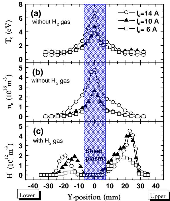
**Fig. 4.** The spatial profiles of (a) the electron temperature T<sub>e</sub>, (b) the electron density n<sub>e</sub>, and (c) the density of H<sup>-</sup> are plotted against the y-direction of width of the sheet plasma.
