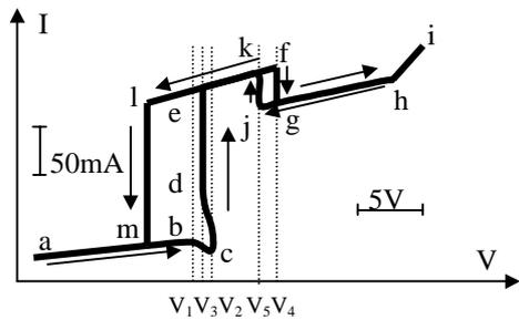
**Fig. 2.** Static  $I(V)$  characteristic of the plasma diode shown in Fig. 1. The branch  $h \rightarrow i$  corresponds to the stimulated strong oscillations in a resonant system coupled to the device.
