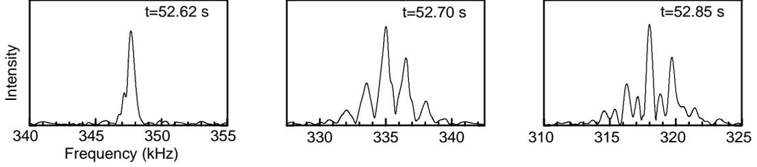
**Fig. 2.** Snapshots of the experimental spectra of magnetic activity for the toroidal Alfvén eigenmode with  $n=7$  in JET discharge #40238.
