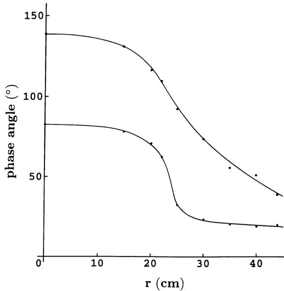
Fig. 3. Profiles of phase difference between  $n_e$  and  $\Phi_D$  oscillations computed with Eq. (2). The upper curve is obtained in a control run where the  $v_{in}$  profile immediately before the gas oscillation is kept and applied during the gas modulation phase.
