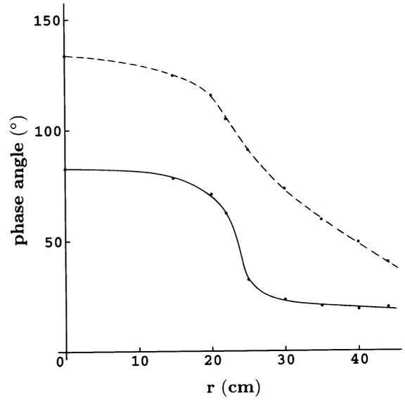
Fig. 2. Profiles of phase difference between  $n_e$  and  $\Phi_D$  oscillations computed with Eq. (1) setting  $C_v = 0.4$  (dashed curve) and with Eq. (2) (solid curve). The minor half-axis of a flux surface is denoted by  $r$ .
