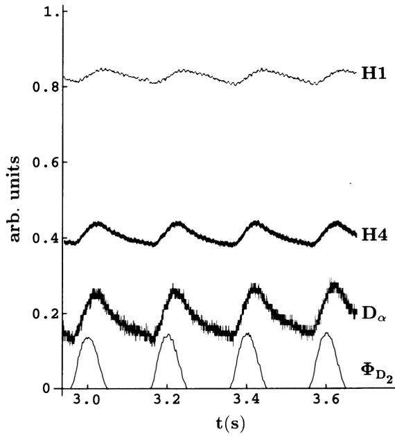
Fig. 1. Temporal evolutions of central and peripheral line average densities H1 and H4, respectively, from DCN interferometry, edge  $D_\alpha$  signal and influx rate  $\Phi_{D_2}$  of deuterium molecules at the gas valve.
