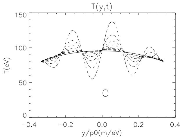
**Figure 5.** Time evolution of the temperature profile in Lagrangian coordinates to the steady state (full line) which corresponds the equilibrium solution in Fig. 6 (b) in Eulerian coordinates.
