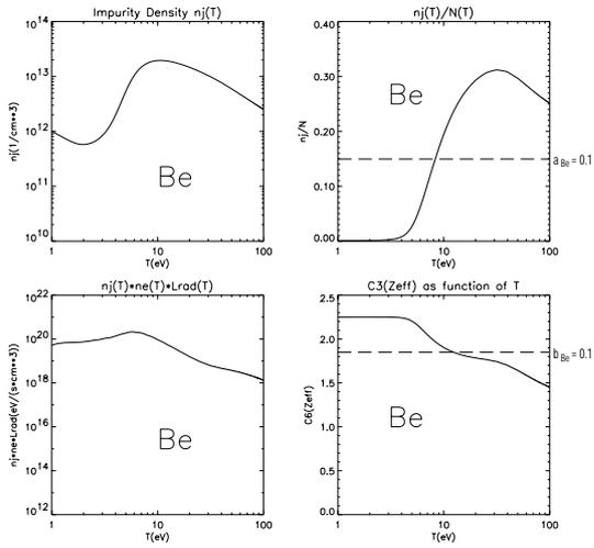
**Figure 3.**  $n_j$ ,  $n_j/N$ ,  $n_j n_e L_{rad}$ ,  $C_3(Z_{eff})$  as functions of  $T$  for Be.
