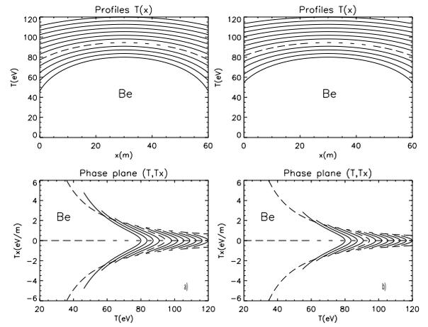
**Figure 4.** Profiles  $T(x)$  and phase plane portraits  $(T, T_x)$  for Be; (a) - exact solution, (b) - SA with  $a_{Be}=0.15$ ,  $b_{Be}=1.85$ .
