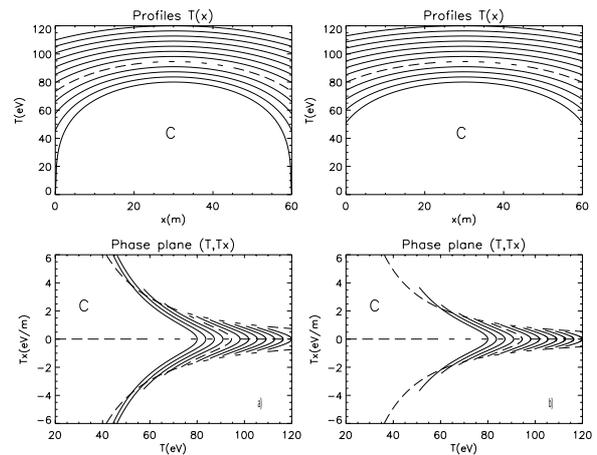
**Figure 2.** Profiles  $T(x)$  and phase plane portraits  $(T, T_x)$  for C; (a) - exact solution, (b) - SA with  $a_C=0.1$ ,  $b_C=1.7$ .
