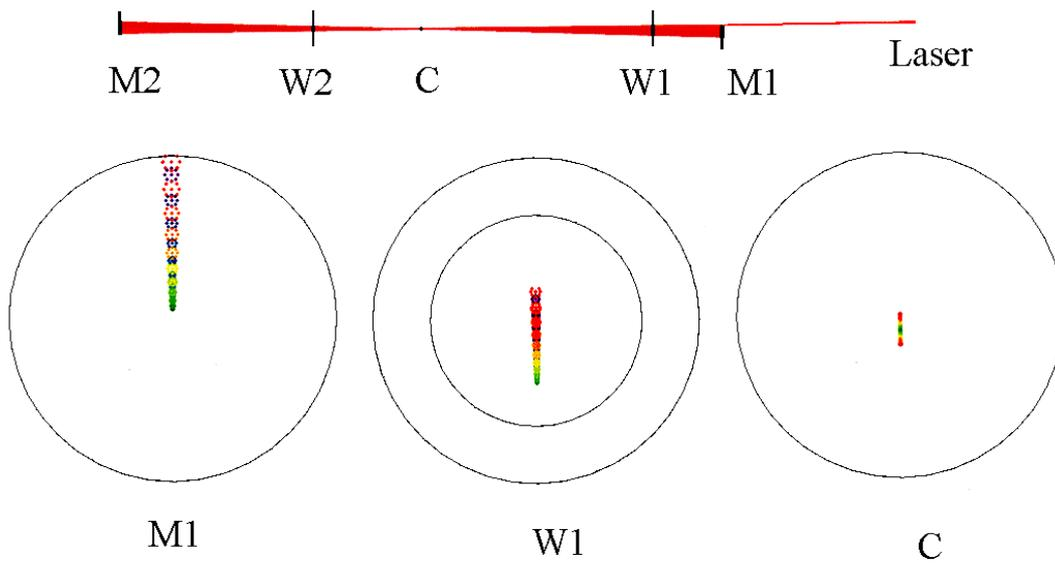
**Figure 2.** Simulation of the ETE multipass injection system (high) with cross sections (low) of the first mirror (M1), window (W1) and plasma center (C).
