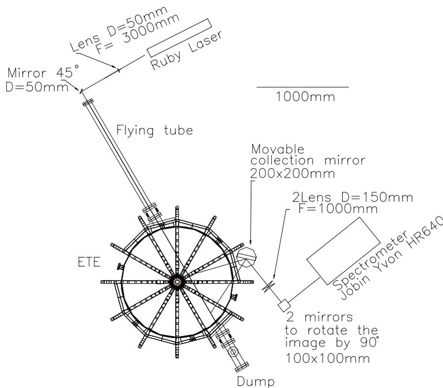
**Figure 1.** Top view diagram of the ETE Thomson scattering system.
