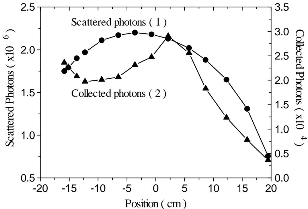
**Figure 3.** Simulation of the collected photons by the system (curve 2 - solid circles) compared with the plasma scattered photons (curve 1 - solid triangles).
