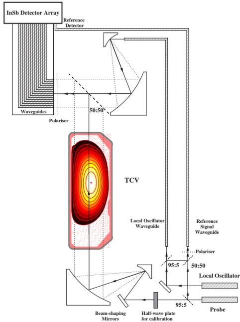
**Figure 1.** Overview of the TCV polarimeter/interferometer
