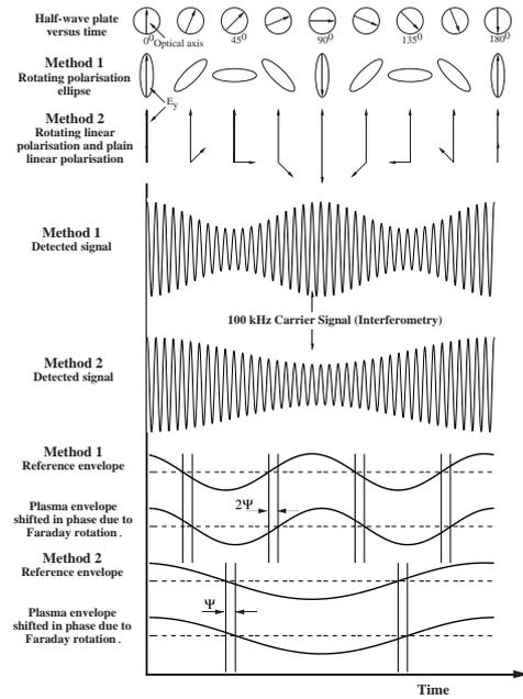
**Figure 2.** Schematic of the two interferometer/polarimeter methods.
