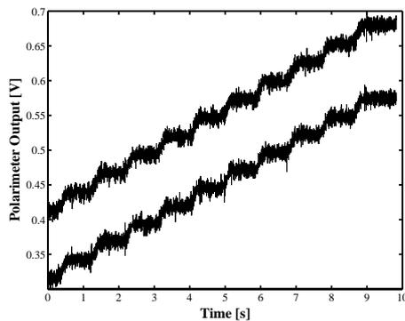
**Figure 4.** Polarimeter output for Method 1 with steps of  $0.4^\circ$  Faraday rotation.
