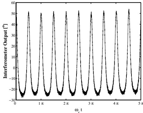
**Figure 6.** Interferometer output for Method 1 with  $\Psi = 40^\circ$  and  $m = 0.48$  where  $\omega_r$  is the rotation frequency of the  $\lambda/2$  plate.
