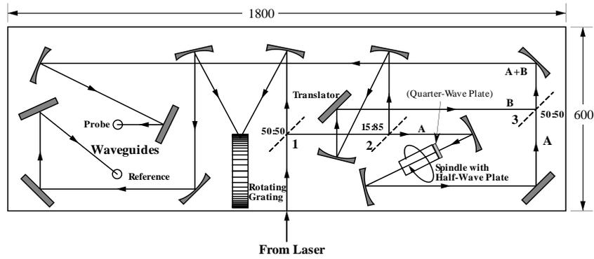
**Figure 3.** The optical set-up for the production of the probe and LO beams.
