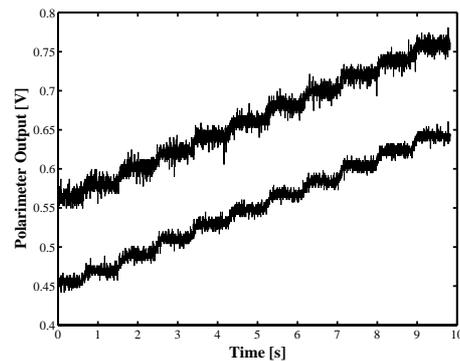
**Figure 5.** Polarimeter output for Method 2 with steps of  $0.4^\circ$  Faraday rotation.
