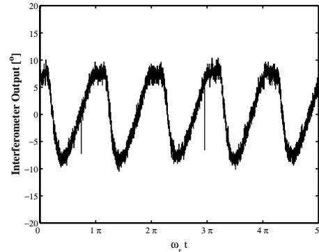
**Figure 7.** Interferometer output for Method 2 with  $\Psi = 40^\circ$  and  $m = 0.4$  where  $\omega_r$  is the rotation frequency of the  $\lambda/2$  plate.
