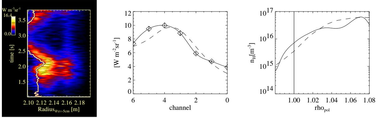
**Fig. 2.** Left:  $H_\alpha$  distribution during a separatrix-shift. middle and right: Comparison of experimental data (diamonds) and data modeled using EIRENE (dashed) (shot #10249).
