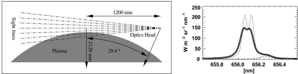
**Fig. 1. Left:** Setup of  $H_\alpha$  diagnostic at ASDEX Upgrade. **Right:** Spectrum; Measured: thick black; Fit: White line inside the thick black line; dotted: Spectral deconvolution; dashed: hydrogen contribution
