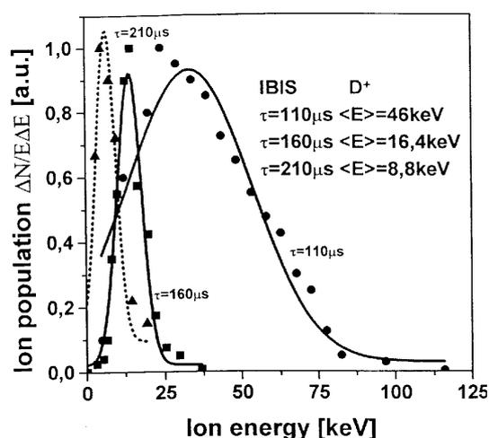
**Fig. 1.** Energy spectra of deuterons from the IBIS facility ( $I_{max} = 600$  kA), as obtained for three different modes of the operation.
