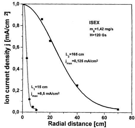
**Fig. 5.** The angular distribution of Xe-ion flux, as measured at a distance of 165 cm and 15 cm from the ISEX outlet, respectively. The data show a divergence of the generated ion streams.
