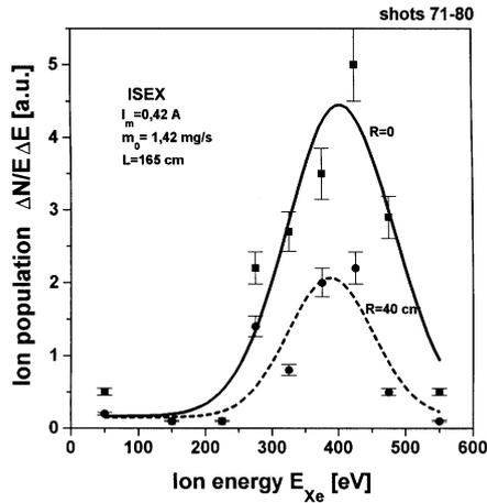
**Fig. 4.** The ion energy spectra of Xe-ions emitted from the ISEX device, as measured with Faraday cups placed at different angular positions. The distance from ISEX to Faraday collectors was  $L = 165$  cm.
