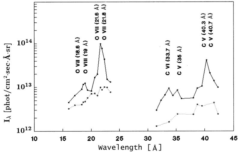
Fig. 2. USX spectrum at 7<sup>th</sup> ms (maximum plasma density-full line) and 3<sup>rd</sup> ms (background-dotted).
