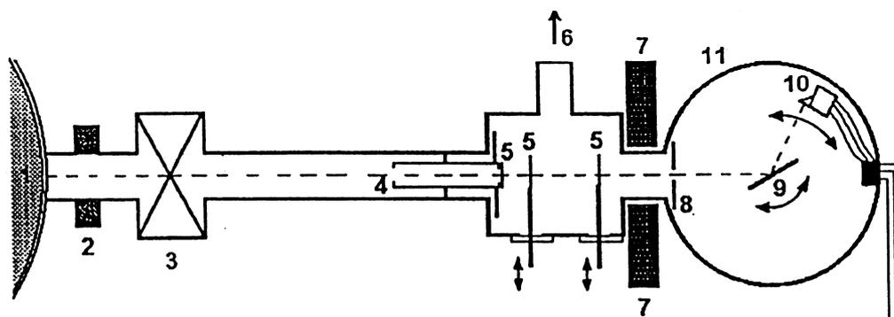
**Fig. 1.** Schematic of the ultra-soft X-ray MLM spectrometer (1-plasma, 2-flange, 3-valve, 4-collimator, 5-filters, 6-pumping, 7-shielding, 8-diaphragm, 9-multilayer mirror, 10-detector).
