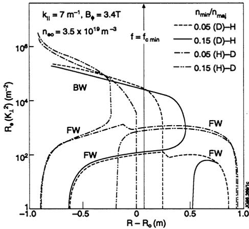
**Fig. 4.** Dispersion diagram for the inverted and normal minority scenarios in a tokamak.
