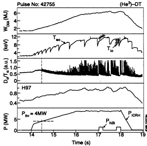
**Fig. 2.** He3-minority (~10%) in a 50:50 DT plasma with strong ion heating ( $T_{i0}=13$  keV)
