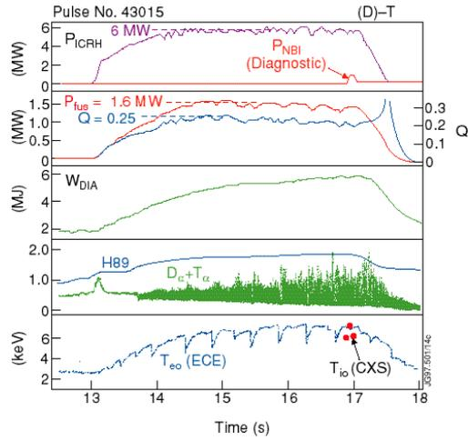
**Fig. 3.** D-minority heating in T-plasma. Non thermal DT neutrons with  $Q \approx 0.25$  for ~ 2s.
