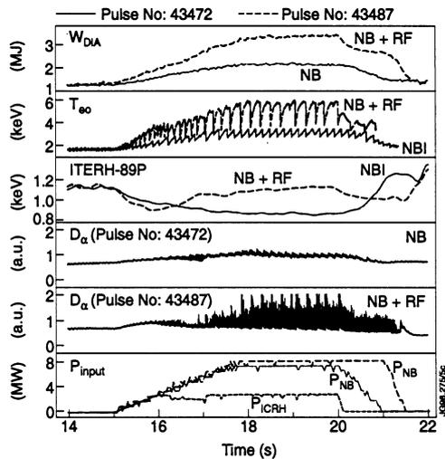
**Fig. 7.** Compare NBI only and NBI+ICRH (inverted (He3)-H discharges).
