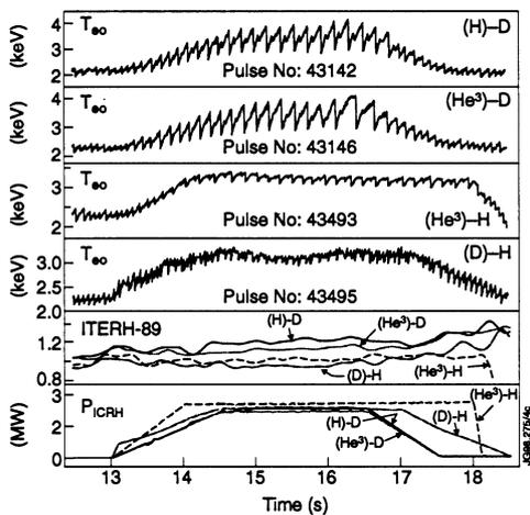
**Fig. 6.**  $T_{e0}$  and confinement factor for normal and inverted minority heating scenarios.
