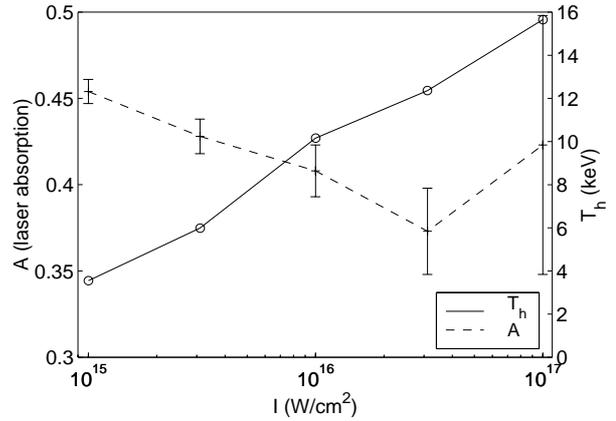
**Fig. 2.** Laser absorption efficiency  $A$  and hot electron temperature  $T_h$  versus laser intensity. P-polarized Nd laser 1.5 ps FWHM Gaussian pulse is incident at  $45^\circ$  on solid Al target.
