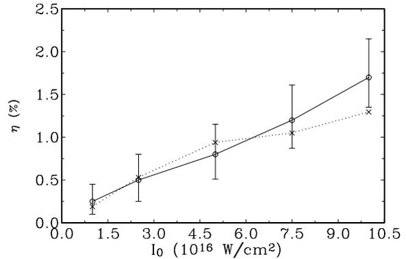
**Fig. 4.** Efficiency  $\eta = I_2/I_0$  of laser energy transformation to SH emission from plasma versus peak laser intensity. P-polarized Gaussian 1.5 ps FWHM pulse of Nd-laser is assumed to be incident at  $45^\circ$  onto a solid aluminium target.
