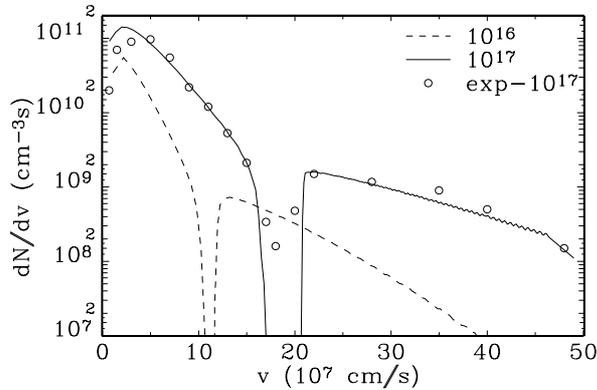
**Fig. 3.** Velocity spectrum of ions at the interaction of 1.5 ps FWHM Gaussian pulse of p-polarized Nd laser radiation incident at  $45^\circ$  on solid Al target for two values of laser intensity.
