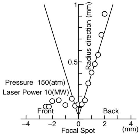
Fig. 2. Calculated light channel and observed radius of plasma.
