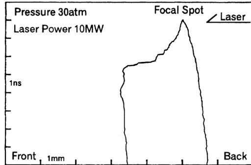
Fig. 1. Typical streak image of the plasma boundary.
