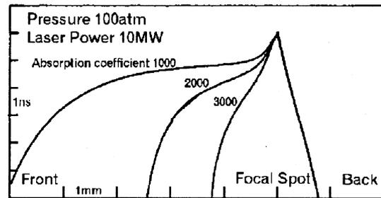
**Fig. 3.** Calculated forward plasma by forward breakdown wave and constant absorption coefficient.
