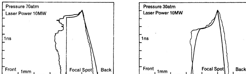
**Fig. 5** Calculated plasma by averaged absorption coefficient and observed plasma.
