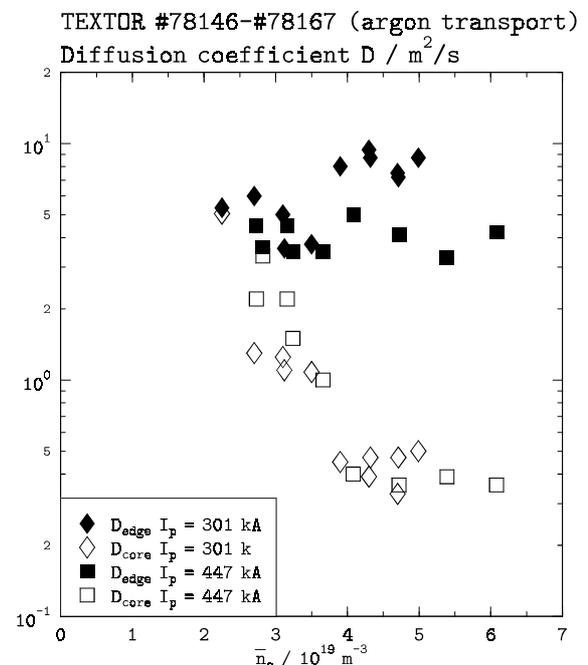
**Figure 4:** Experimental results evaluated by STRAHL calculations: diffusion coefficients for plasma edge and core at different mean densities and plasma currents
