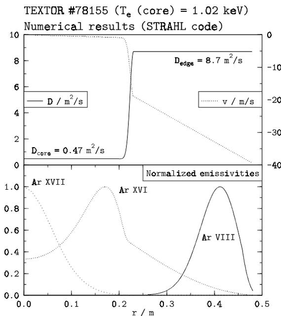
**Figure 3:** (upper graph) Radial profiles of diffusion coefficient  $D$ , radial drift velocity  $v$  of argon; (lower graph) argon emissivity profiles calculated by STRAHL
