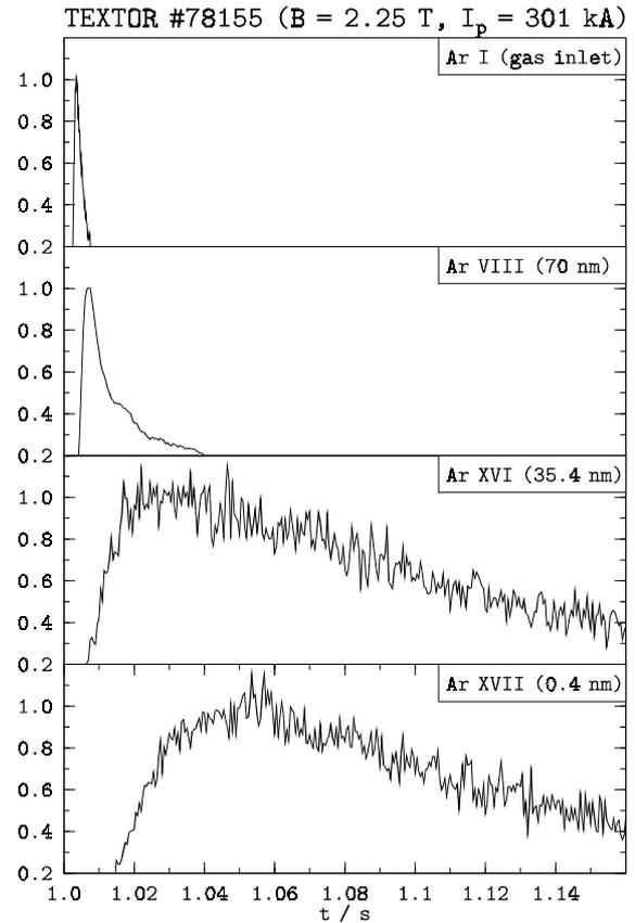
**Figure 2:** Measured normalized argon line intensities after a gas puff at  $t = 1.0$  sec.
