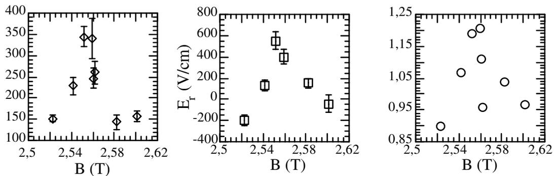
**Fig. 2:** Left: central ion temperature, middle: central radial electric field, right: inverse density profile peaking factor for He III. All versus the magnetic field strength measured at  $r = 1.6\text{ cm}$ .
