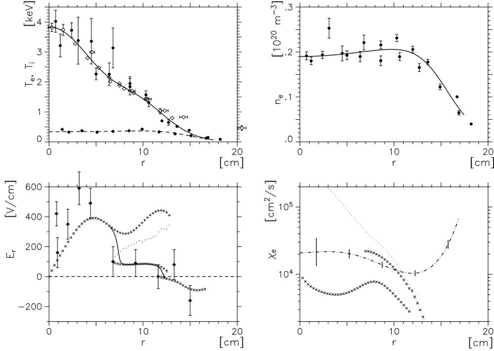
**Figure 1:** Upper left: electron temperature (solid line), ion temperature (broken line). Upper right: electron density. Lower left: radial electric field (dots: CXRS, crosses and points: neoclassical calculation). Lower right: electron heat balance (dot-dashed: experimental, crosses and points: neoclassical calculation).
