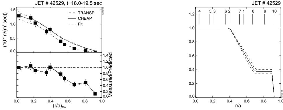
**Fig. 2:** Left: Measured and predicted 2.5 MeV brightness profile with and without correction to beam-thermal emissivity, Right: Radial function used to correct the beam-thermal emissivity. The closest approach of the line of sight for the channels of the horizontal camera is marked.
