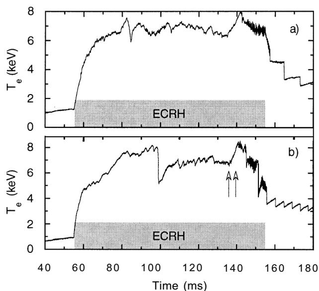
**Fig. 1.** Time traces of  $T_e(0)$  for FTU pulses: a) #12608 with  $P_{\text{ECRH}} = 293$  kW and b) #12799 with  $P_{\text{ECRH}} = 360$  kW. The arrows mark the times for the profiles shown in Fig. 2.
