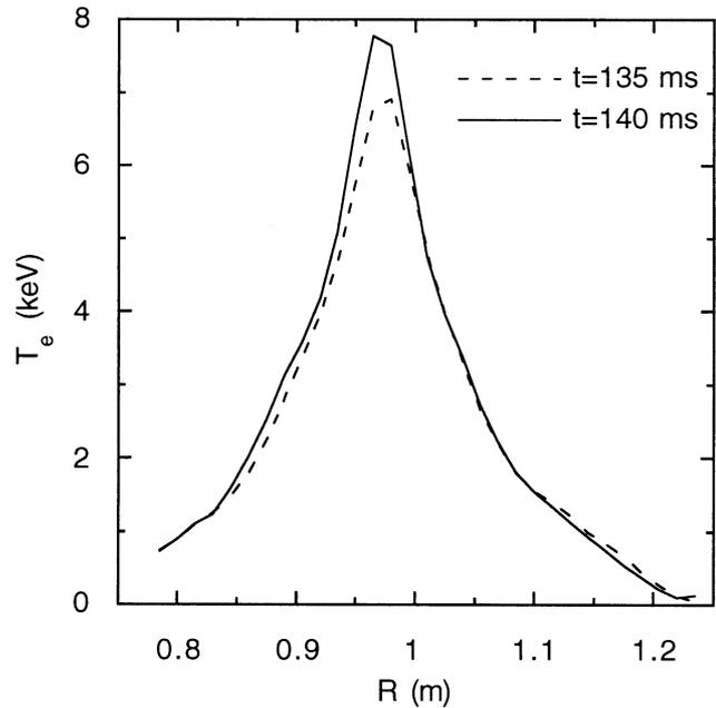
**Fig. 2.** Temperature profiles before and during the  $T_e$  rise at  $q_{\min} \approx 1$  for FTU pulse #12799.
