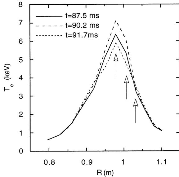
**Fig. 4.**  $T_e$  profiles during the fluctuation at  $q_{\min}=2$  in FTU pulse #12660. The arrows mark the positions of the channels shown in Fig. 3.
