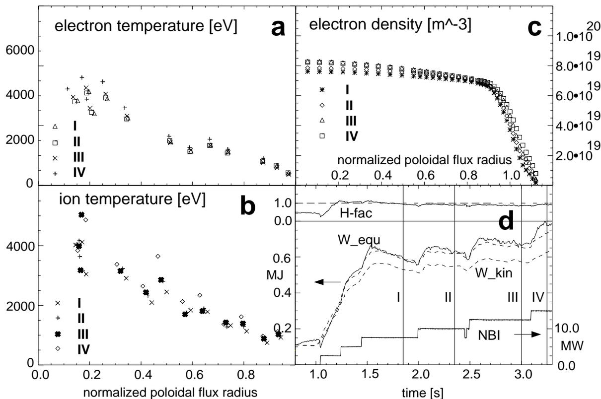
**Figure 5.** High power medium density discharge in deuterium (#10397, 1 MA, 2.0 T)
