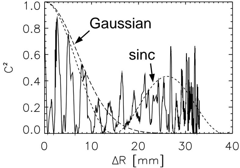
Fig. 1: Correlation  $C^2$  versus distance  $\Delta R$  between the cut-off layers (solid line) approximated by a Gaussian curve (broken line) and sinc-functions (dotted line).
