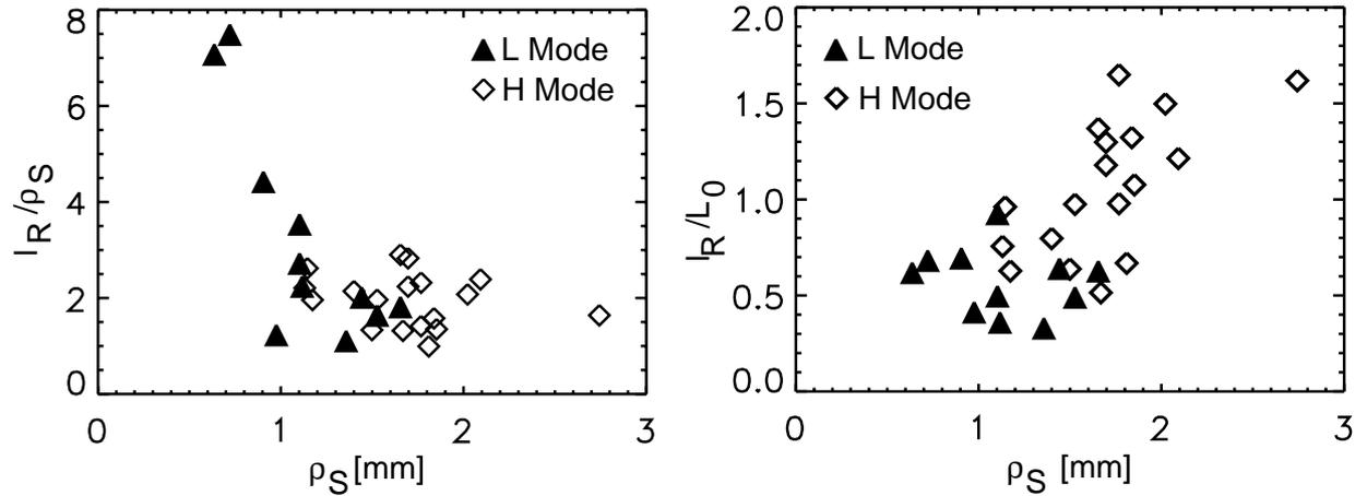
Fig. 3: Scaling of the radial correlation length  $l_R$  normalized to the effective gyroradius  $\rho_S$  and normalized to  $L_0$  versus  $\rho_S$ .
