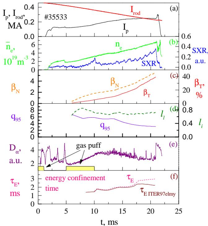
**Fig. 1.** Traces of a high- $\beta$  shot #35533.  $30\text{kV}$ ,  $\sim 0.9\text{MW}$  hydrogen neutral beam was applied from the beginning of the discharge into a deuterium plasma.
