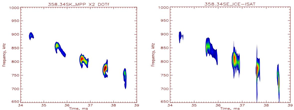
**Fig. 5.** Outer midplane Mirnov coil and Langmuir probe spectrogram from shot #35834.
