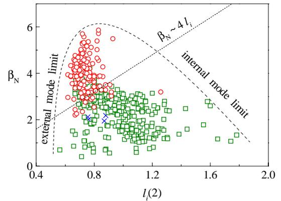
**Fig. 3.** Stability diagram in  $\beta_N$  vs  $l_i$  space for START. Each point represents one shot. Stability limits (qualitatively) expected from conventional tokamak experience are shown.
