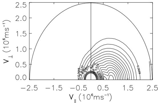
**Fig. 4.** Contours of velocity distribution,  $F_b(v)$  of fast NBI ions sampled at plasma core determined by the LOCUST NBI Monte Carlo code [4]. Non-monotonic  $\partial F_b/\partial v$  is generated at the plasma centre by virtue of large poloidal flux excursion and high propensity for charge exchange in the plasma periphery.
