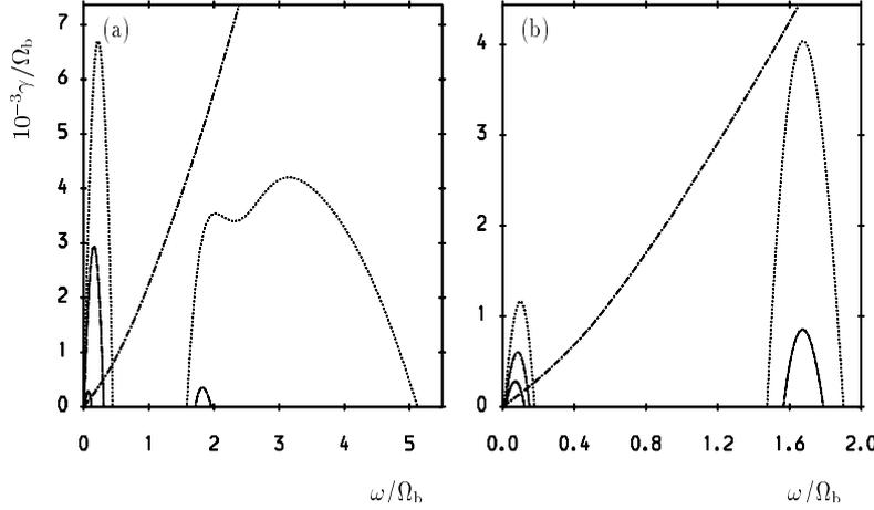
**Fig. 6.** Computed growth rates of fast Alfvén waves in START, showing the effect of varying (a)  $v_{\perp}/c_A$  and (b)  $\delta v_{\perp}/v_{\perp}$ . In (a)  $\delta v_{\perp}/v_{\perp}=0.3$  and  $v_{\perp}/c_A=3$  (solid curve), 3.25 (dashed curve), 3.5 (dotted curve). In (b)  $v_{\perp}/c_A=3$  and  $\delta v_{\perp}/v_{\perp}=0.3$  (solid curve), 0.28 (dashed curve) and 0.26 (dotted curve). The dashed-dotted curves show electron damping.
