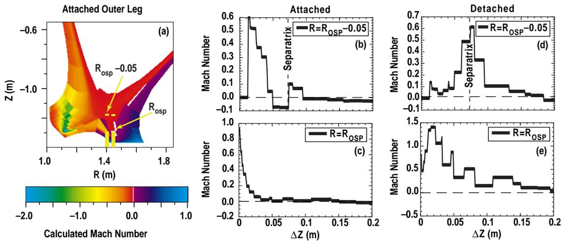
Fig. 2. The 2-D calculations of Mach number obtained by UEDGE, and two paths meant to simulate those taken by the probe are shown (a). Calculated Mach number for cuts along those paths crossing the separatrix (b) and entering the SOL directly (c) are shown for attached discharges. Calculated Mach number for the same paths (d–e) are also shown.
