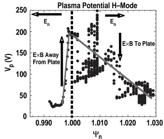
Fig. 3. Plasma potential profile (V) plotted versus normalized flux  $\psi_n$ . The separatrix is at  $\psi_n=1$ . The electric field is of the order of 200 V/cm.
