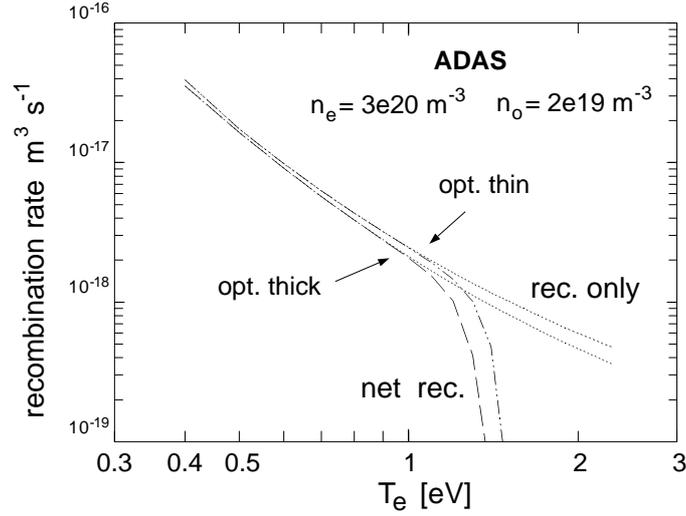
**Fig. 2:** Recombination rate coefficients (including net rates) for optically thin and thick conditions
