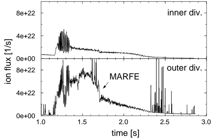
**Fig. 4:** Plasma fluxes to the inner and outer divertor target measured with Langmuir probes
