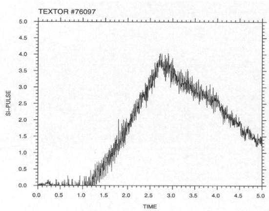
**Figure 2:** Typical silane puff into the TEXTOR-94 plasma as determined by the SiII line radiation.
