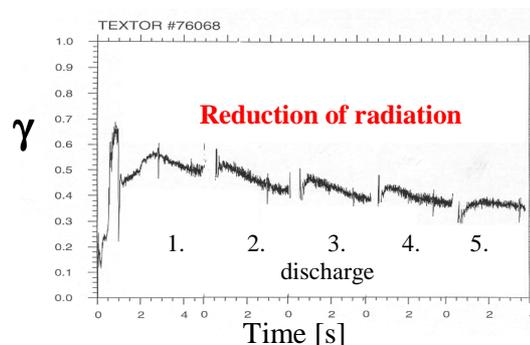
**Figure 4:** Reduction of the fraction  $\gamma$  of radiated power vs. total heating power after the turn off of the silane injection. (Several discharges are compiled in one figure.)
