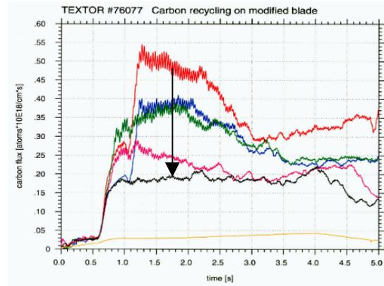
**Figure 1:** Reduction of the carbon flux recycling at the ALT-II limiter due to multiple injection of silane in subsequent discharges.
