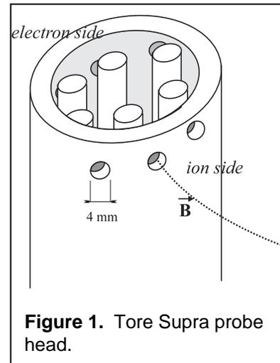
**Figure 1.** Tore Supra probe head.
