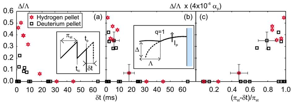
Figure 2: (a)  $\Delta/\Lambda$  vs.  $\delta t = t_{lc} + \pi_{st} - t_p$ . (b)  $\alpha_p \Delta/\Lambda$  vs.  $\delta t$ . The factor  $\alpha_p$  takes into account the differences between the initial pellet parameters.  $\Delta$ ,  $\Lambda$  and  $\delta t$  are described in the two insets. (The factor  $4 \times 10^{-6}$  is for the convenience of the display.) (c)  $\alpha_p \Delta/\Lambda$  vs.  $(\pi_{st} - \delta t)/\pi_{st}$ .
