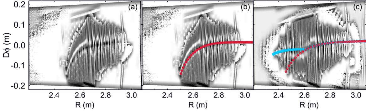
Figure 1: [Pellet TS12635] (a) Reprocessed time-integrated CCD image of the ablation pattern . The pellet is injected from right to left in the tokamak midplane.  $D\phi$  is the toroidal direction and  $R$  the major radius. (b) Same picture with the calculated trajectory superimposed (red markers). [Pellet TS12637] (c) The trajectories are calculated with the current densities displayed in Fig. 3b: unperturbed trajectory (red markers), perturbed trajectory (blue markers).
