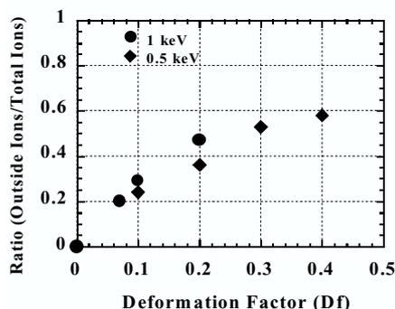
Fig.6 Dependence of radial drift on deformation factor.
