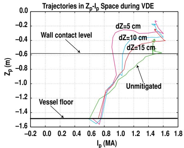
Fig. 5. Trajectories in  $Z-I_p$  space for varying vertical positions at which gas injection occurs. The fraction of plasma current lost by the time of wall-impact is greater the earlier the injection is performed.
