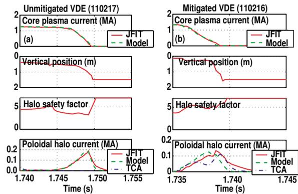
Fig. 3. Application of halo model to unmitigated (a) and mitigated (b) discharges shows good agreement for  $T_e(\text{unmitigated}) = 5$  eV,  $Z_{\text{eff}}(\text{unmitigated}) = 1.5$ ,  $T_e(\text{mitigated}) = 2.4$  eV,  $Z_{\text{eff}}(\text{mitigated}) = 1.5$ .
