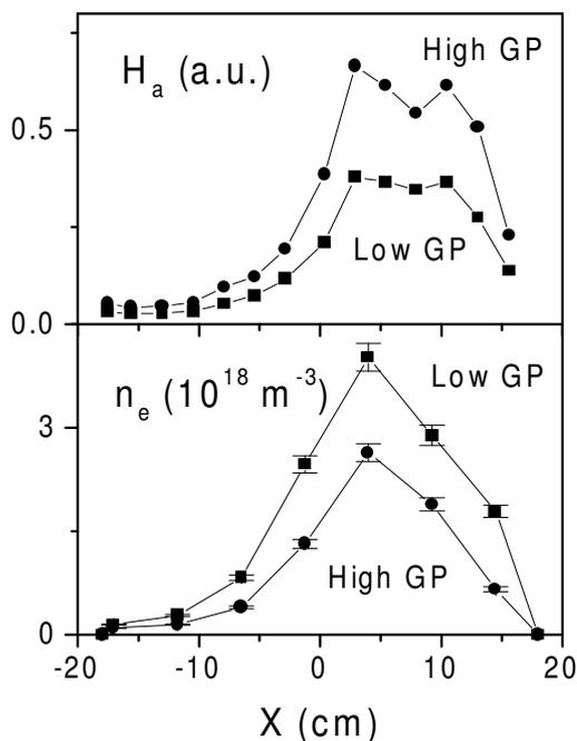
Fig. 2. Radial profiles of plasma density and  $H_{\alpha}$  emission.
