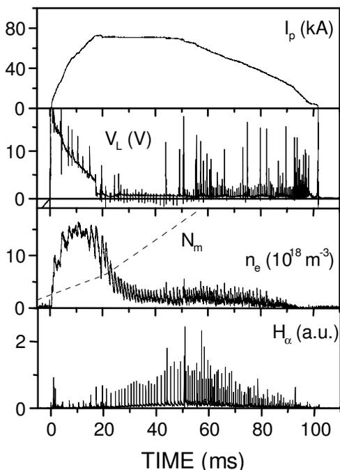
Fig. 1. Runaway discharge with high neutral density;  $N$  is neutral density due to gas puffing.
