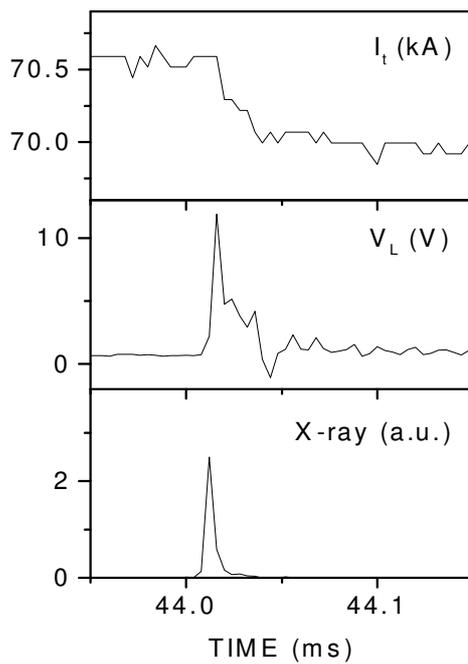
Fig. 3. Spikes in toroidal current and loop voltage caused by runaway losses.
