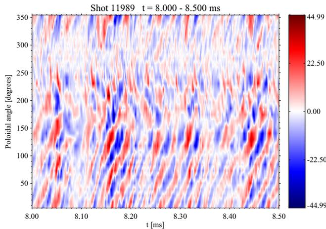
Fig. 2: Floating potential fluctuations plotted as a function of time and poloidal angle.
