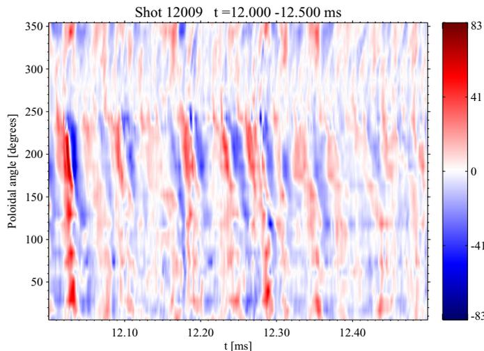
Fig.6: Floating potential fluctuations, plotted as a function of time and poloidal angle, during edge biasing.
