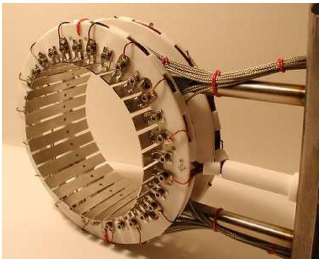
Fig.1: Poloidal array of electrodes and probes.
