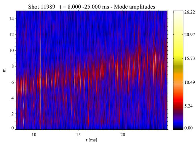
Fig. 4: Time evolution of the mode amplitudes in a discharge with ramping-down plasma current.
