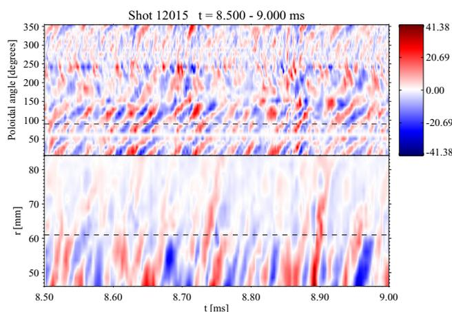
Fig. 5: Top: floating potential fluctuations plotted as a function of time and poloidal angle. Bottom: floating potential fluctuations plotted as a function of time and radial position. The dashed lines mark the intersection of the two arrays.
