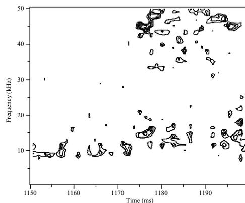
Fig 6 - Plot of the spectrum of a Mirnov coil (shot 5127). A 43 kHz mode is activated at  $t \approx 1173$  ms, when the cold pulse front arrives at  $\rho = 0.3-0.4$ .
