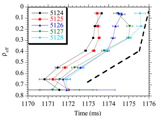
Fig 5 - Time of arrival of the cold pulse front, seen with the ECE diagnostic. The dashed line corresponds to propagation at 10 m/s for  $\rho > 0.4$  and at 80 m/s for  $\rho < 0.4$ .
