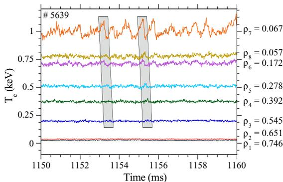
Fig 3 - ECE electron temperature traces showing the propagation of heat pulses.
