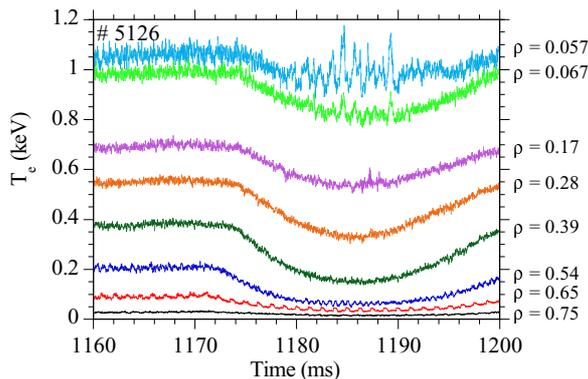
Fig 1 - ECE electron temperature traces for discharge 5126.
