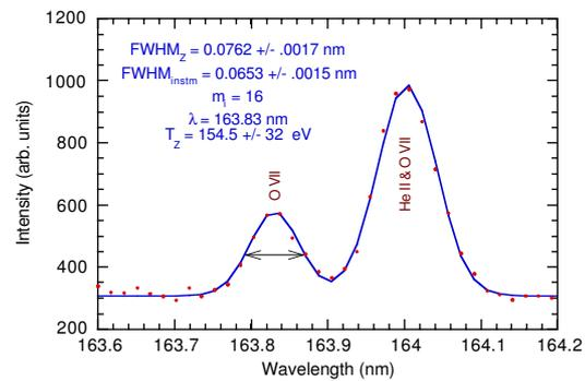
Fig. 2. Gaussian fit to O VII lines
