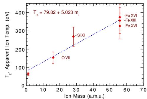
Fig. 3: Apparent Doppler ion temperatures as a function of emitting ion atomic mass.
