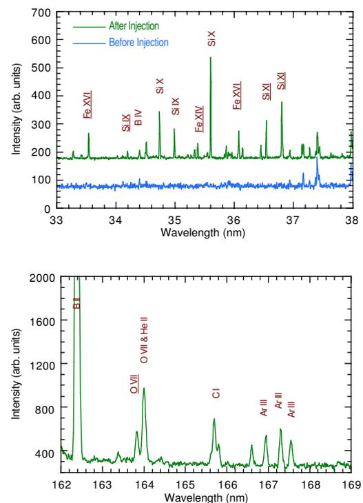
Fig. 1. TJ-II spectra of a) emission before and after laser ablation was performed. (The Si and Fe lines considered for determining Doppler temperatures are underlined), and b) the O V II emission line (also underlined).
