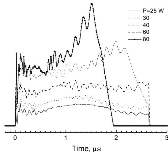
**Fig. 6.** Reflected microwave pulses after homodine detection for different pump power.
