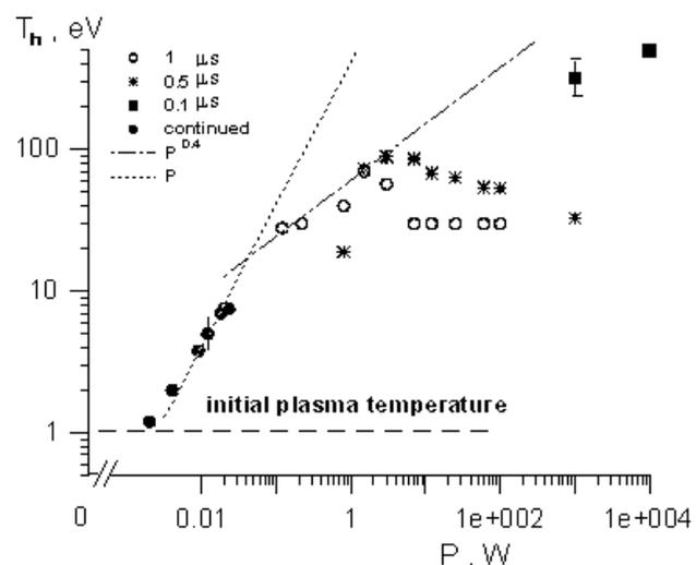
**Fig. 3.** Dependence of electron effective temperature on the pump power.
