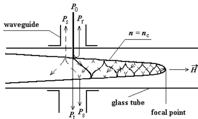
**Fig. 1.** The scheme of EPW excitation and propagation.
