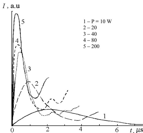
**Fig. 5.** Waveforms of accelerated electron current for different pump power.
