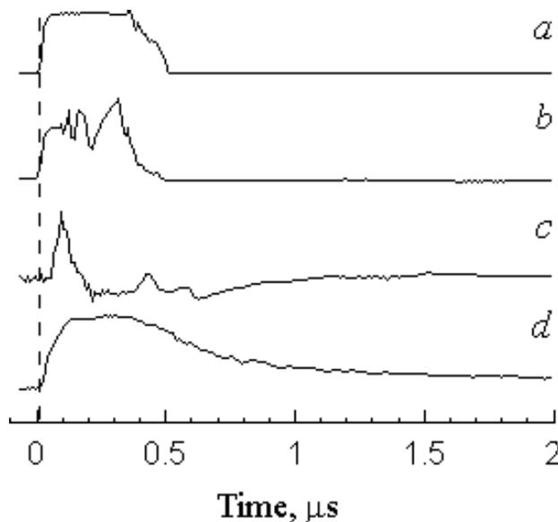
**Fig. 2.** Oscillograms of incident (a), reflected (b) microwave pulses, electron current (c) and plasma luminosity(d).
