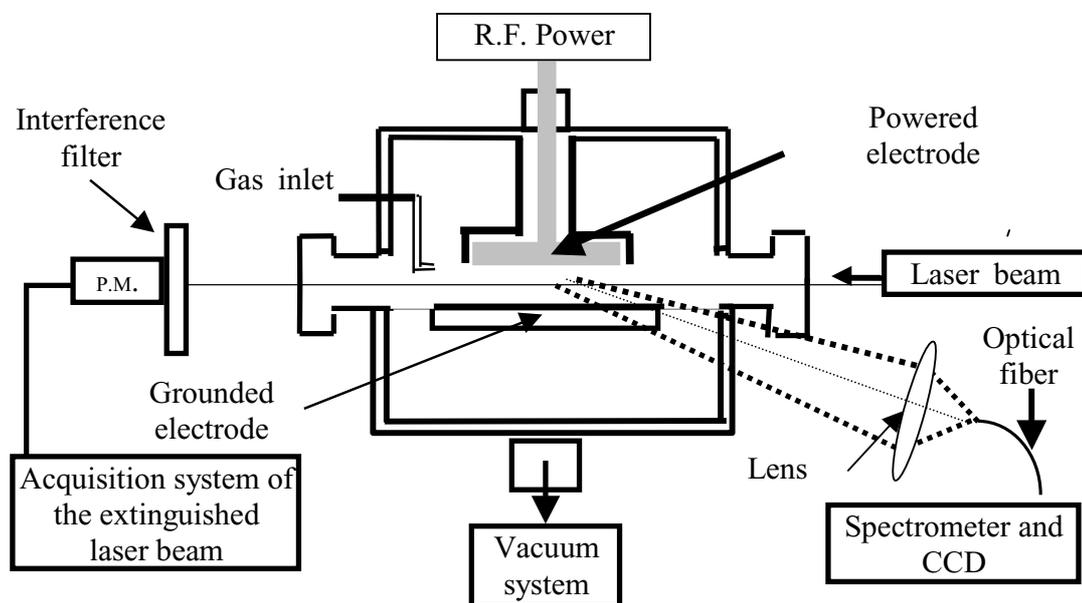
Figure 1 : Experimental set-up
