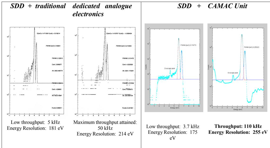
Fig 2.2: Results obtained with an  $^{55}\text{Fe}$  radioactive source
