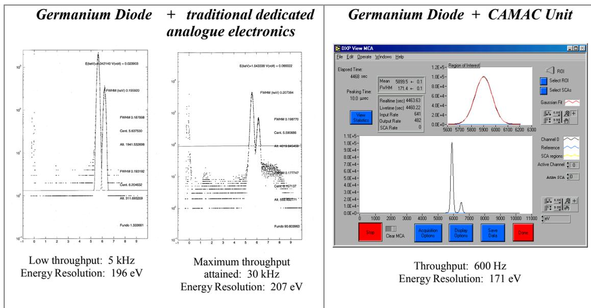
Fig 2.1: Results obtained with an <sup>55</sup>Fe radioactive source
