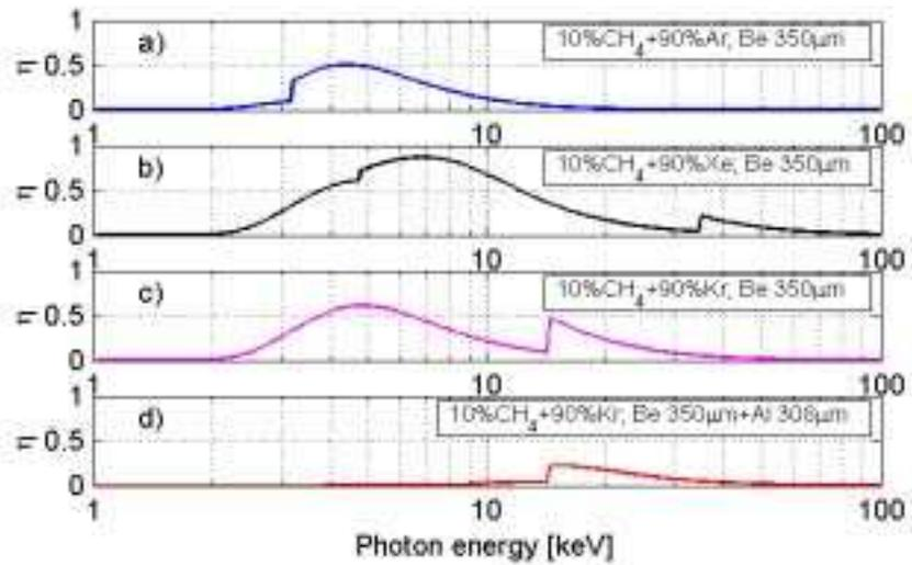
Fig. 2 Overall spectral sensitivity of the MPX diagnostic for different gas mixtures and foils.
