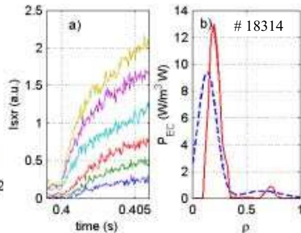
Fig. 6 X-ray intensity time traces ECH switched on  $t=0.4$  s (a); ECH power deposition profiles (solid line TORAY, dashed COBRA) (b).
