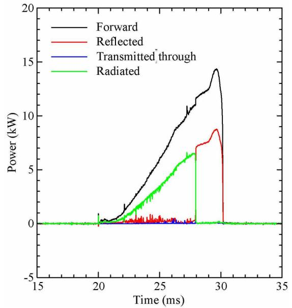
Fig. 2. Forward, reflected, transmitted, and radiated power for antenna launching waves in the lower hybrid range of frequencies
