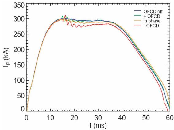
Fig. 1. Toroidal plasma current with different phasing of applied oscillating poloidal and toroidal loop voltages
