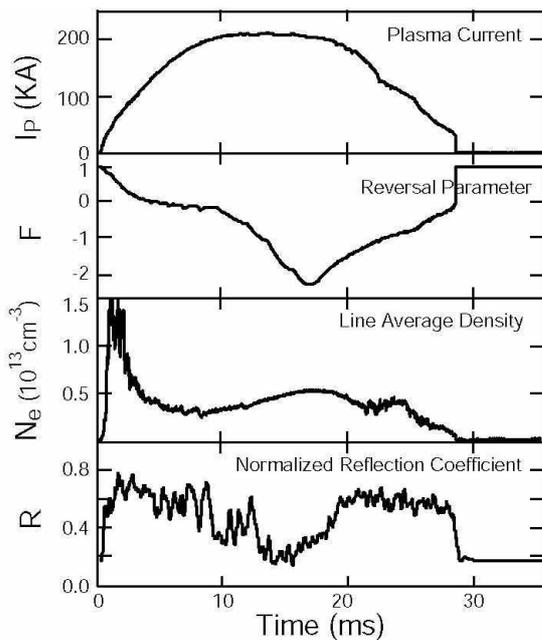
Fig. 3. Plasma current, reversal parameter, line-averaged density, and reflection coefficient for single waveguide launching power in the electron cyclotron range of frequencies
