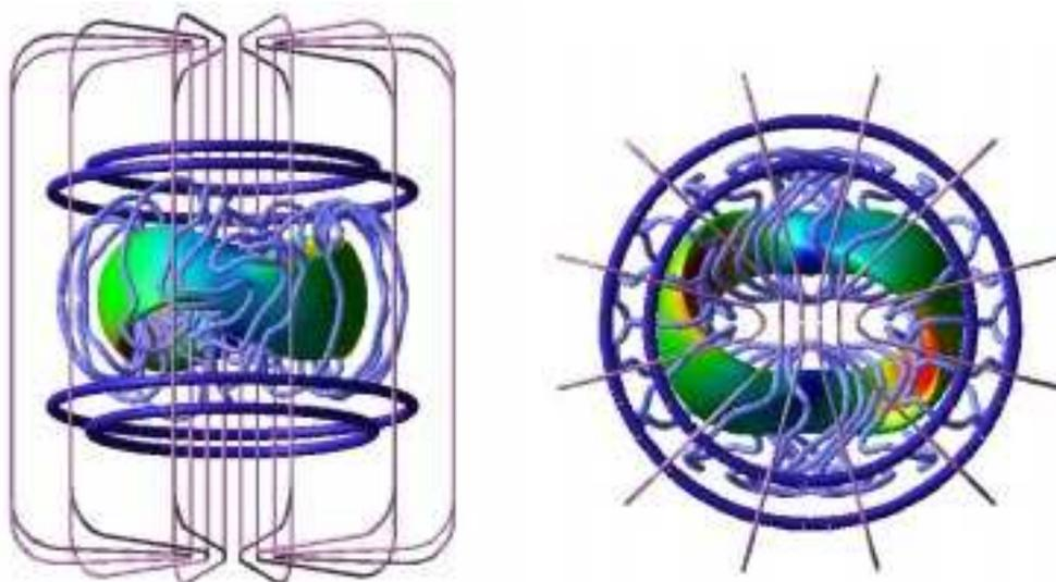
*Fig. 1. (a) Side and (b) top views of outer magnetic flux surface and the three coil sets (modular, vertical, toroidal) with color contours showing magnetic field strength.*
