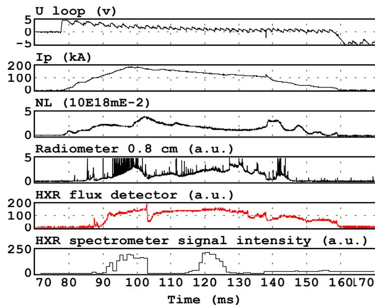
Fig.1 Experimental waveforms of plasma parameters in very low density discharge #3577. From top to bottom: loop voltage, plasma current, line-averaged density, intensity of 0.8cm radiation recorded by radiometer, HXR intensity by flux detector, integrated over energy spectrum HXR intensity
