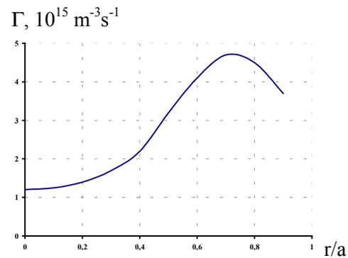
Fig.4 Radial dependence of runaways production rate for the low density discharge #2657
