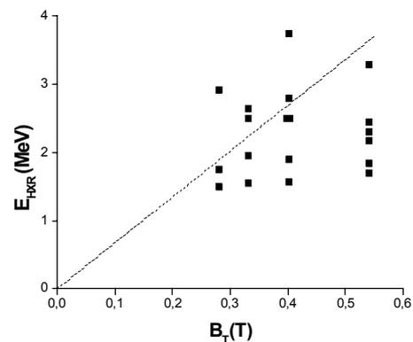
Fig.3 Dependence of maximum runaways energy on toroidal field strength for moderate densities
