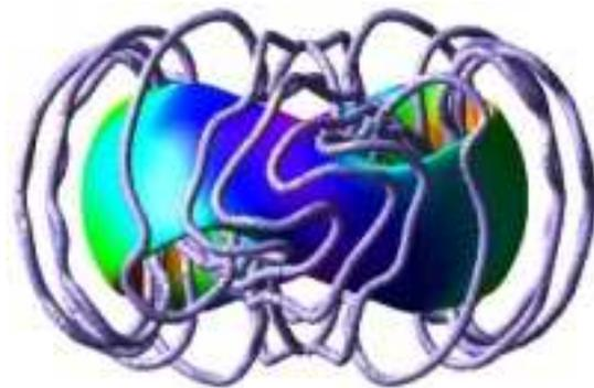
Fig. 1. Top (left) and side (above) views of the QPS plasma and the optimized modular coil geometry used to create it. The colors indicate contours of constant  $|B|$  in T on the last closed flux surface.
