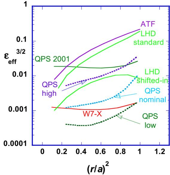
Fig. 4. Coefficient of thermal diffusivity in the  $1/\nu$  regime for different stellarators and the variation possible in QPS.
