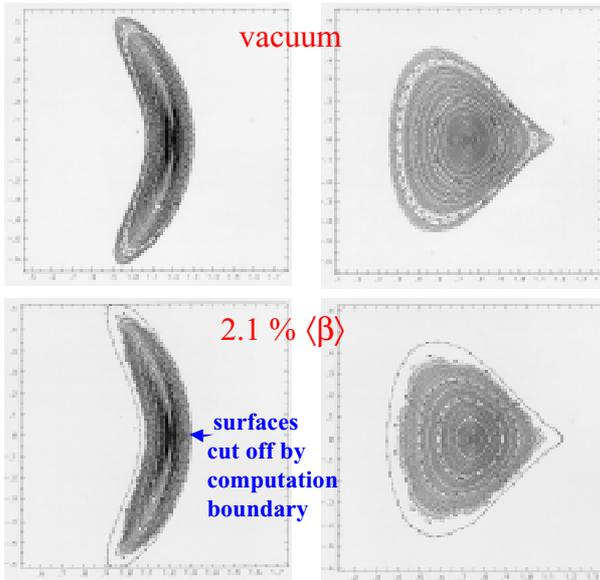
Fig. 5. Magnetic surfaces at the symmetry planes for vacuum and  $\langle \beta \rangle = 2.1\%$ .
