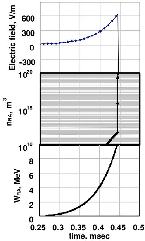
Fig3. The runaway generation in the thermal quench with inclusion of the secondary avalanching (time points marked by arrow) in large tokamak.
