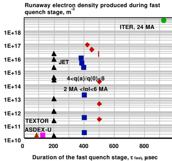
Fig5. The runaway generation in the thermal quench without inclusion of the secondary avalanching (upper values of the runaway density are pre-avalanche values for JET and ITER)
