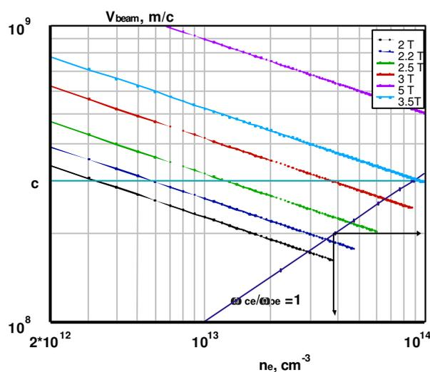
Fig.1a. The runaway instability criterion (2) on the accessible values of the  $V_{beam}$  plotted vs. plasma density.
