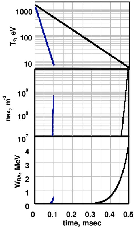
Fig.2. The runaway generation in the thermal quenches with different times of fast quench for medium size tokamak experiment
