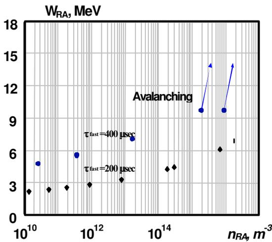
Fig.4. The runaway generation in the thermal quenches with different times of fast quench in large tokamak (JET,  $4 < q(a)/q(0) < 8$ ,  $2 \text{ MA} < I_{pl} < 6 \text{ MA}$ ,  $\langle n_e \rangle = 10^{20} \text{ m}^{-3}$ )
