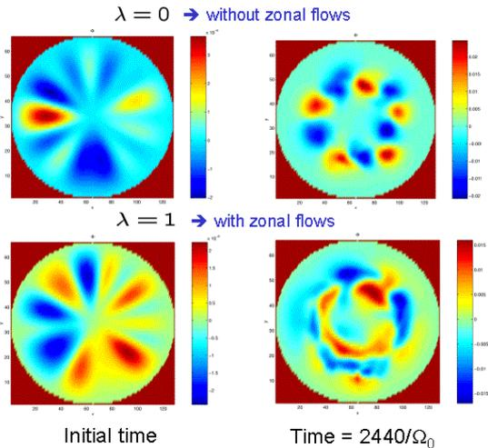
Figure 4: Cross-section of the electric potential in  $(r, \theta)$ , at initial time and time in the saturation phase ( $t=2440/\Omega_0$ ), for both cases  $\lambda = 0$  and  $\lambda = 1$ .
