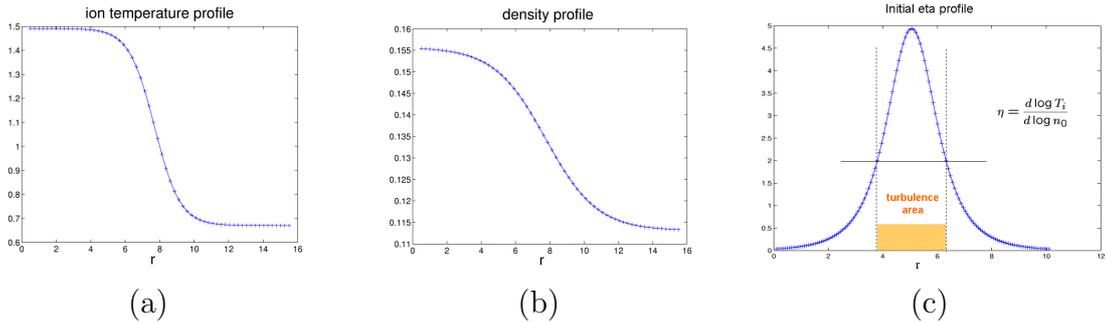
Figure 2: (a) Ion temperature profile :  $T_i(r)$ . (b) Density profile :  $n_0(r)$ . (c)  $\eta_i$  profile.
