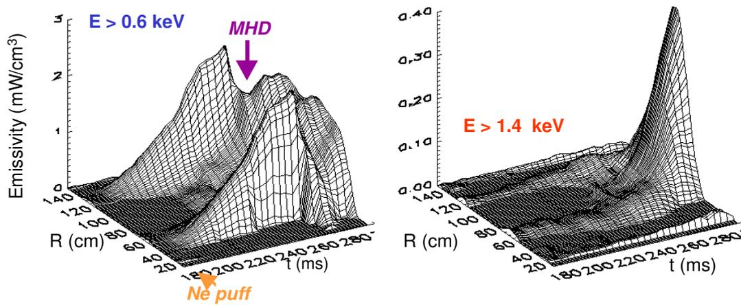
**Figure 2.** Evolution of the Ne emissivity in the  $E > 0.6$  keV and  $E > 1.4$  keV spectral ranges
