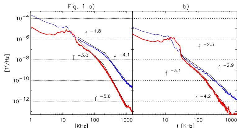
ensemble average over 1 ms intervals taken between  $t=9$  ms and  $t=18$  ms, i.e. in the period where plasma current remains stationary.
