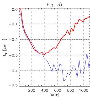
the toroidal correlation length). A particularly interesting quantity is the first moment of  $S(k,\omega)$ , i.e. the statistical dispersion relation  $\bar{k}_\phi(\omega) = \int dk \frac{k}{2\pi} (S(k,\omega)/S(\omega))$  of the magnetic turbulence. Results for standard (blue) and PPCD (thick red) 0.4 MA ensembles are shown in Fig. 3 (similar results hold for 0.5 MA): we observe a marked difference for frequencies in excess of 300-400 kHz
