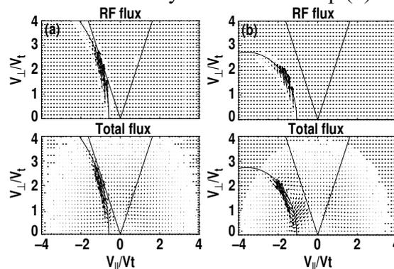
Fig. 4. The flux in velocity space due to the wave-particle interaction (upper panels) and the total flux including collisional effects (lower panels) calculated by CQL3D for two cases: (a) low  $\beta_e$  ( $n_{e0} = 2 \times 10^{19} \text{ m}^{-3}$ ,  $T_{e0} = 4 \text{ keV}$ ) and (b) higher  $\beta_e$  ( $n_{e0} = 6 \times 10^{19} \text{ m}^{-3}$ ,  $T_{e0} = 12 \text{ keV}$ ). In both cases  $p = 0.385$  and poloidal angle is near  $90^\circ$ .
