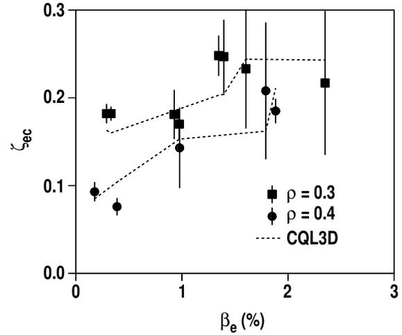
Fig. 2. The measured normalized current drive efficiency as a function of  $\beta_e$ , for  $\rho=0.3$  (squares) and  $\rho=0.4$  (circles) [4]. In all cases the poloidal angle is near  $90^\circ$ . The dotted lines represent the results of calculations for the experimental conditions.
