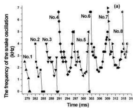
**Fig.2a** The frequency evolution of the pellet-induced snake oscillation
