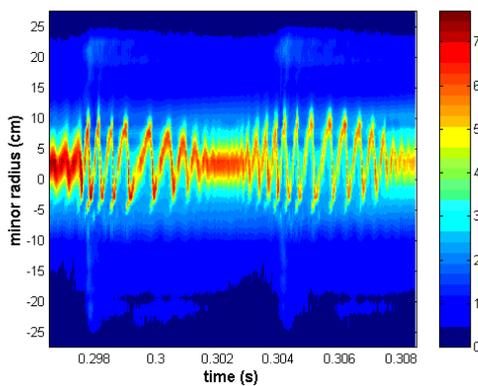
**Fig.1** The time evolution of the pellet-induced snake on the SXR radiation signal
