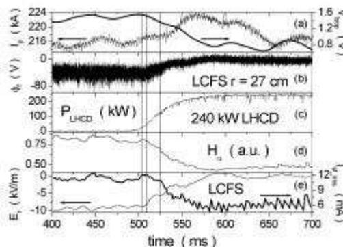
Fig.5: The related changes of  $I_p$ ,  $V_p$ , edge floating potential ( $\phi_f$ ),  $H_\alpha$  intensity, edge  $E_r$ , probe's saturated ion current after the onset of LHCD in the discharge as in Fig.3.
