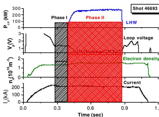
Fig.3: The plasma energy confinement times are 14.6ms (H=1.16) and 24.5ms (H=2.11) in phase I (without LHW) and phase II (with LHW) respectively.
