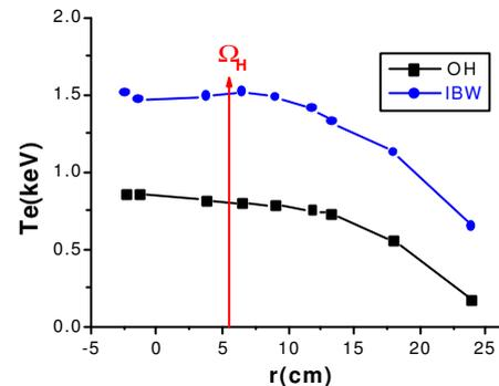
Fig.7: The comparison of  $T_e$  profiles w/o IBW in a discharge. The H<sup>+</sup> resonance layer is close to the center.
