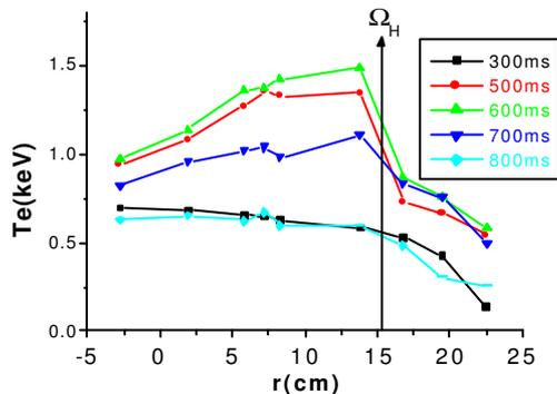
Fig.6: The evolution of electron temperature profile in an IBWH discharge. The profiles at 300ms and 800ms were taken just before and after IBWH. Electrons in the zone near H<sup>+</sup> resonance layer were clearly heated.
