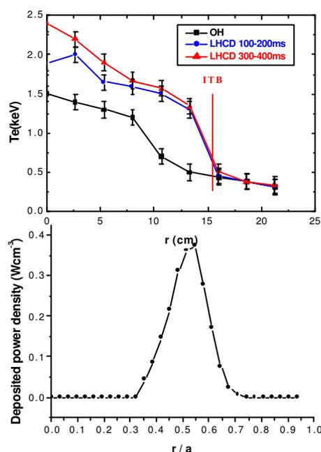
Fig.4: Above are the  $T_e$  profiles measured by soft X-ray spectrometers in the discharge as in Fig.3; The below is the calculated LHCD deposition profile.
