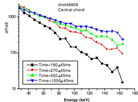
Fig.8: Central channel hard X-ray spectra from a LHCD and IBWH discharge. The black one was taken at the time (180ms) only with LHCD. The color ones were taken with the two waves together.
