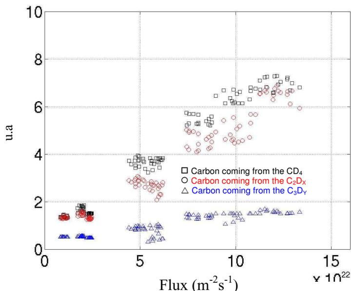
Fig. 2 : carbon production versus incident deuterium ions flux for each ohmic shot.
