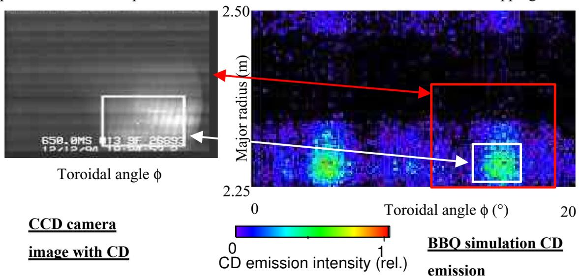
Fig. 3 : Comparison of the BBQ simulation of CD emission from a segment of the toroidal pumped limiter, with a CCD camera image of CD emission
